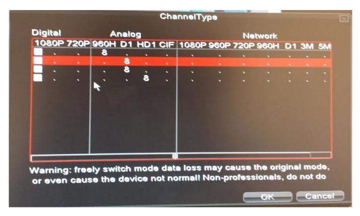
Next, set the corresponding recording type for each camera. Go to Main Menu > Record. Set the resolution to the same setting (Either 960H or D1) that you selected in the Channel Type menu. Click "Application" to save, and the process ir complete.
