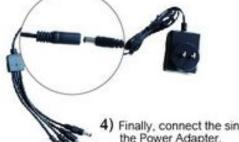
Repeat step 2 with all cameras until all cameras are connected to available channels at the rear of the DVR and all cameras red (female) power connectors are connected to all available black (male) connectors on the 4-Port Power Splitter(s).
