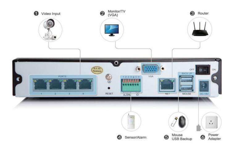
1. Make sure that your router is securely connected to the NET port on the NVR (ZP-NE14-S) using an ethernet cable. The NVR will be unable to locate the any cameras that are connected to it unless the NVR is also connected to a router.
