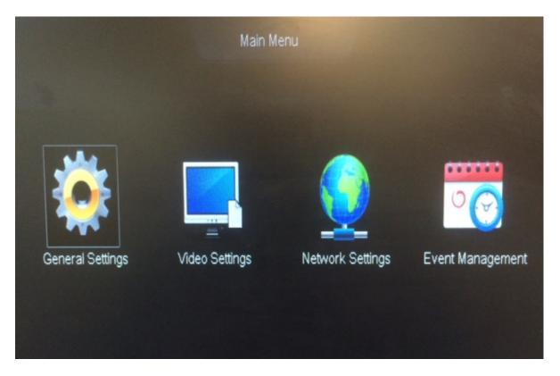
From the general settings menu, click on "PTZ settings" from the left column. There you can enter the info from your PTZ camera. Basic settings require the channel, protocol, baud rate, and address in order for the camera to move on command.
