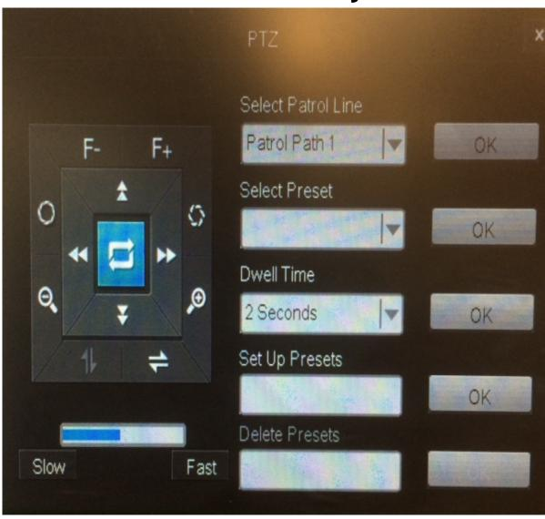
Using this controller, you can move the camera to the desired position, enter numbers between 1-16 in the "Set Up Presets" field to program "Patrol Path 1". Once you have the presets entered, click OK next to "Patrol Path 1" and the camera will begin the tour. "Patrol Path 2" uses presets 17-32.
