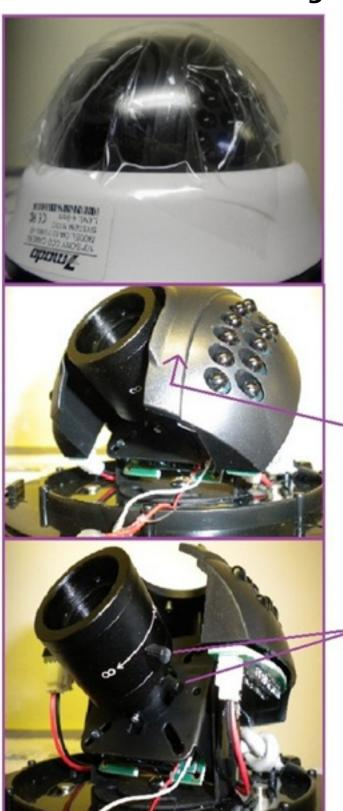
To remove the clear plastic dome cover, simply anchor the bottom plate of the camera and gently twist the white plastic section counter-clockwise.
