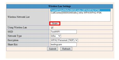
16. Type your WiFi password in the "Share Key" field and then click submit. The screen will change and start a 30 second countdown. Remove the ethernet cable with 20-25 seconds left.
