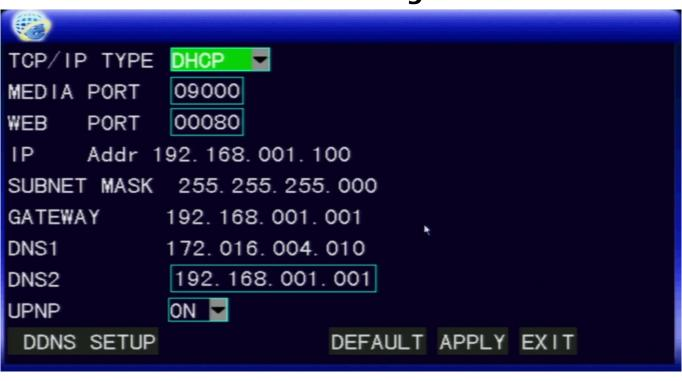
2) Once the DVR boots back up, go back in to the Network Settings and write down the IP address, Gateway (router's IP), and all port numbers. Keep this information for the Remote Network Setup.
