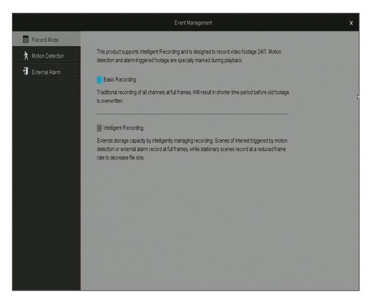
If you pick Basic Recording, the NVR will record 24 hours a day, seven days a week on all channels at the highest possible framerate. If you pick Intelligent Recording, the DVR will record at the full 30FPS when the NVR detects motion, but when there is no motion the NVR will only record one frame every 5 seconds. This is a really good way to make sure you're covering all necessary recordings while maximizing HDD space.
