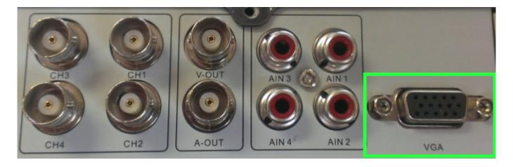
If the cable is plugged in properly, then you must try to reset the resolution to defaults.
