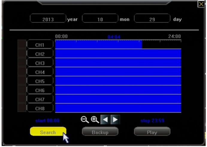
After the desired day has been set and you have clicked search the grid in the middle will have the video for that 24 hour period loaded in to it. From left to right the grid goes from midnight(start of day) to midnight(end of day). The horizontal bars are broken down by channel. In order to see video footage you will select a Page 2/4
