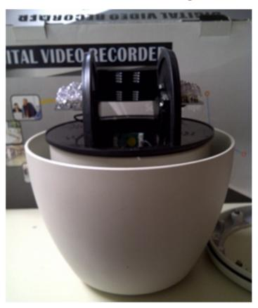
2. Once the inner housing appears to be completely seated and centered inside of the outerhousing, mount the outer housing cover just enough to hold the cover on.
