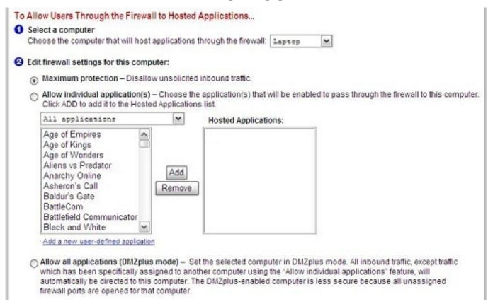
First, look for the DVR's IP address under (1) Select a computer. If you do not see the DVR's IP address here, you may need to go in to the DVR's Network Settings, and set the DVR to DHCP (instead of Static), then reboot the DVR. Once the unit reboots, check it's IP address in the Network Settings, then go back to your router to select the DVR from the list.
