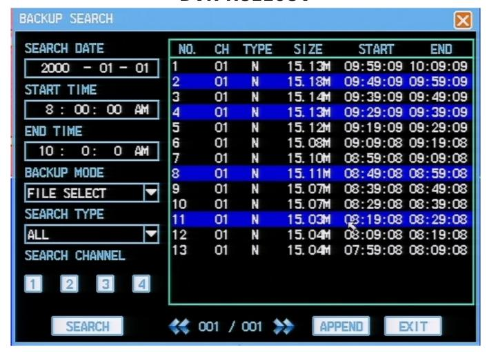
From top to bottom, in the backup search window, fill out the date, start time, and end time of the files you are looking for. Be sure to change backup mode to "File Select". You may narrow down the type of files returned with the search type(to display only files of regular record or motion record types).
