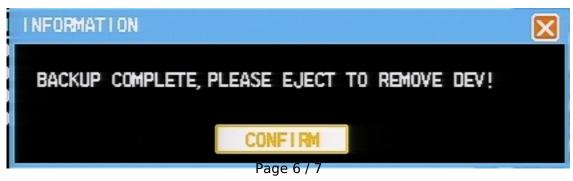
Press confirm. You will be returned to the backup screen one final time. From here select the "Remove" option, and then you may remove the USB flash drive from the DVR.
