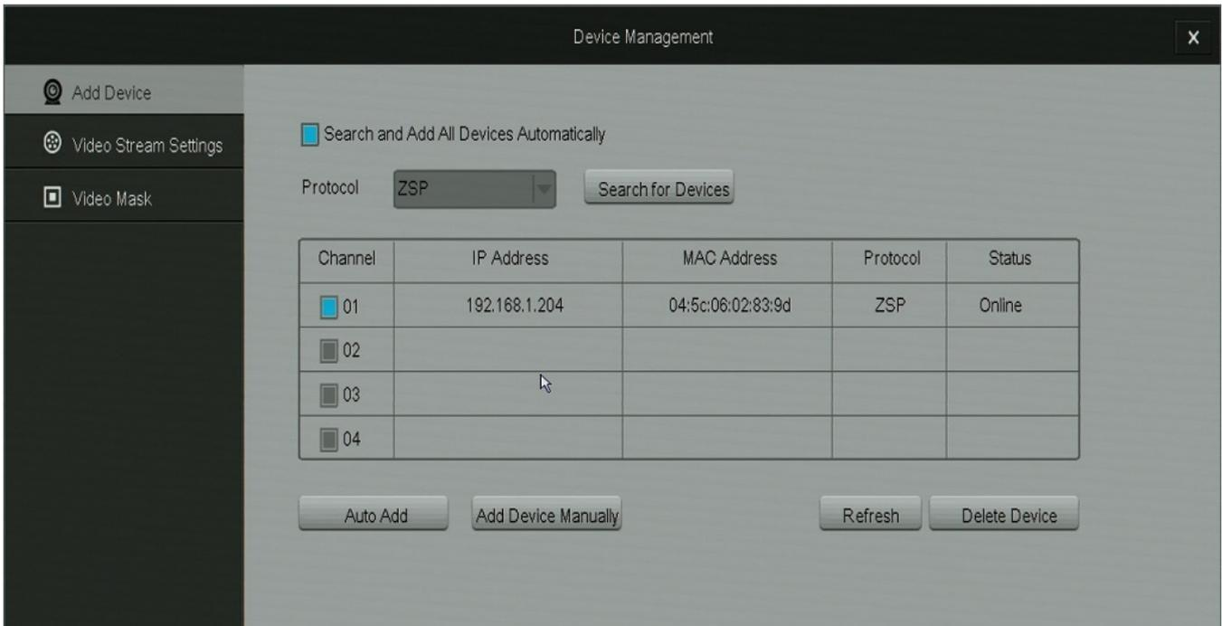
Here you can copy down the IP addresses and see which channels they are currently connected to. Select the camera you wish to change using the box under "channel" and delete the cameras as needed. You can then select "ADD DEVICE MANUALLY"
