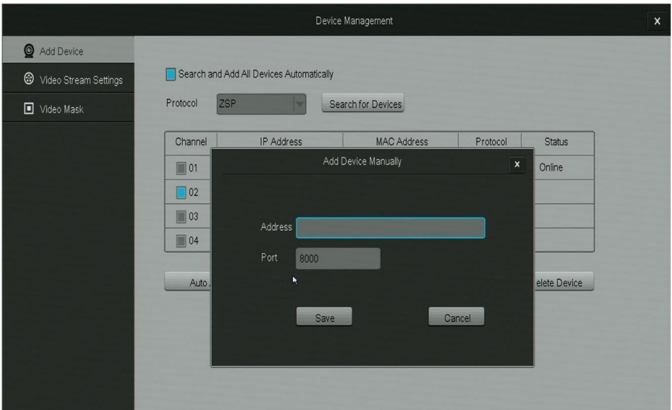
You can enter the IP address of the camera you wish to add in the order that you want them to be listed. Although you can not directly select which channel the camera will connect to, the system will order them starting with channel 1.
