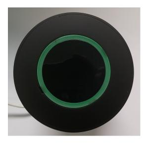
**Solid Green:** The Pivot is booting, you w **Blinking Green:** The Pivot is ready and w during the setup, and anytime the Pivot is
