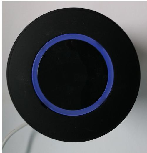
**Solid Blue:** The Pivot is connected to WiFi and the connection is complete.
