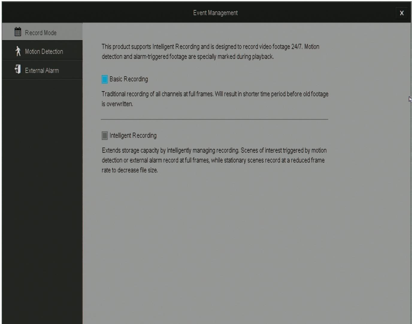
If you pick Basic Recording, the NVR will record 24 hours a day, seven days a week on all channels at the highest possible framerate. If you pick Intelligent Recording, the DVR will record at the full 30FPS when the NVR detects motion, but when there is no motion the NVR will only record one frame every 5 seconds. This is a really good way to make sure you're covering all necessary recordings while maximizing HDD space.
