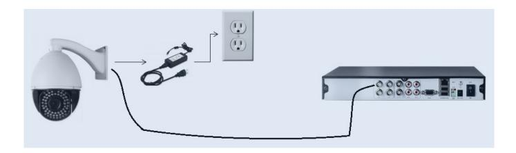
Another option if your cameras need to be between 150ft - 1,000ft from your DVR location, is to use Video Baluns to run the video from your DVR. Video baluns can convert a video signal to a balanced signal, allowing the signal to transfer over Cat5 cable up to approximately 1,000ft. Power will still need to be plugged directly into the camera from a shorter distance.
