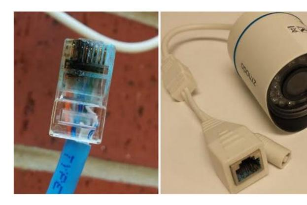
To weatherproof the cable ends, you can either tape the cable ends or install the cable ends into a conduit box. By far the safest option is to install the cable ends into a conduit box to protect the cable ends from the rain and wind.
