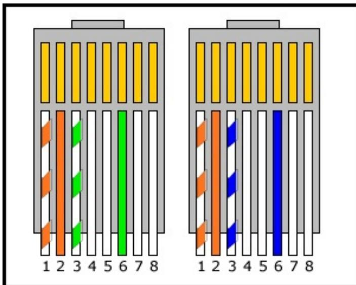
Pinout on SPOE cables included in the kit.
