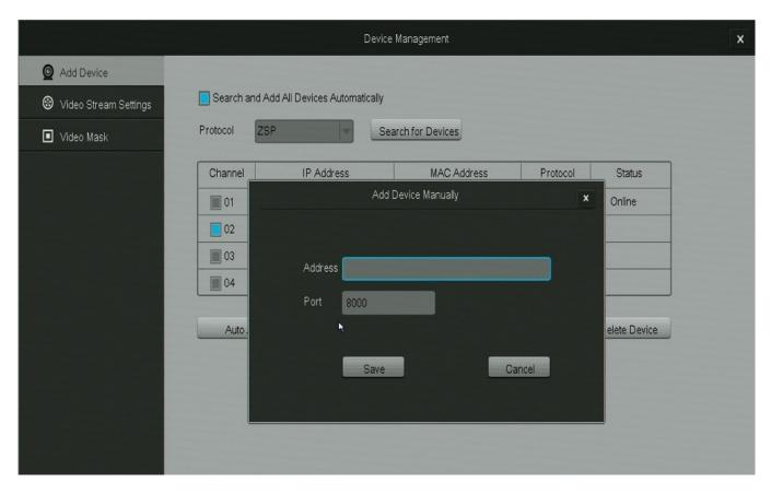
You can enter the IP address of the camera you wish to add in the order that you want them to be listed. Although you can not directly select which channel the camera will connect to, the system will order them starting with channel 1. Unique solution ID: #1354
