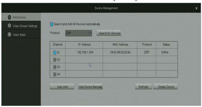
Here you can copy down the IP addresses and see which channels thay are currently connected to. Select the camera you wish to change using the box under "channel" and delete the cameras as needed. You can then select "ADD DEVICE MANUALLY"
