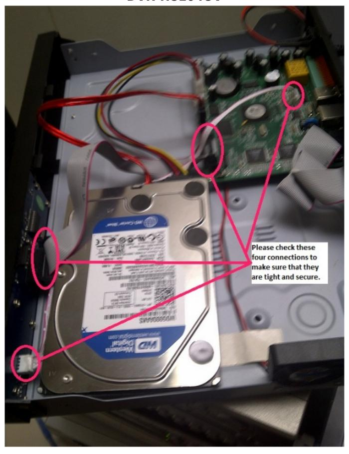
If any of these cables are lose or disconnected, this would cause the video image to Page 2 / 3
