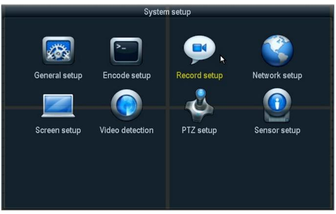
In the record setup menu the first thing to do will be to set the Channel to 1 and the weekday to "Everyday". Next we will put a check mark in the "Motion" box on the "Schedule1" line and remove any other checkmarks we see. Schedule1 should be set to "00:00 - 23:59". Finally in the bottom left we will set the "Copy to" line to All and then press the "Copy to" button. Finally you will press "Ok".
