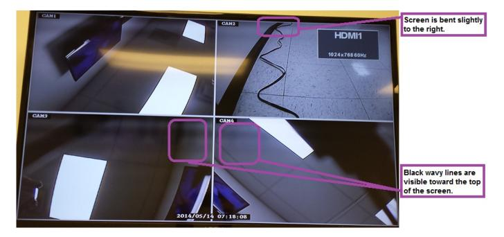
The DVR requires a software update to the March 2014 software build in order to fix this issue. Please complete the following steps in order to upload the correct software to the DT-SFN6:
