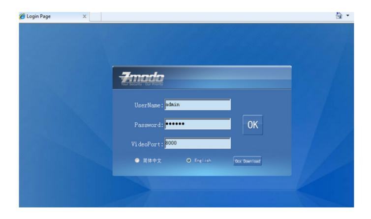
Once you log into the camera with the username: "admin" and password: 111111, click on the gear tap on the top and then select "Remote Configuration".
