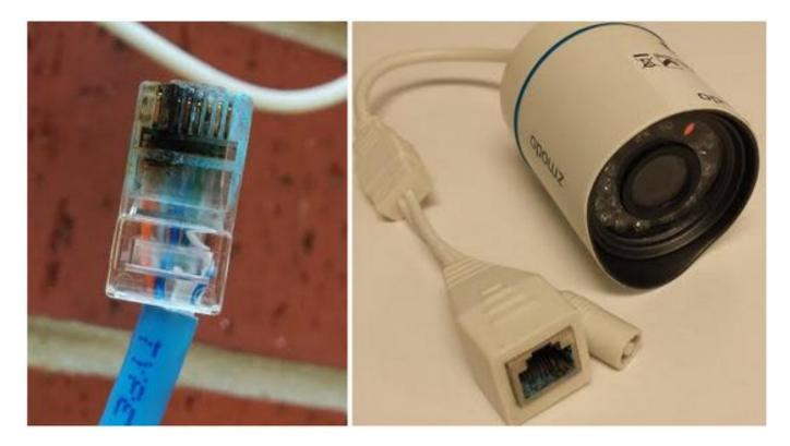
To weatherproof the cable ends, you can either tape the cable ends or install the cable ends into a conduit box. By far the safest option is to install the cable ends into a conduit box to protect the cable ends from the rain and wind.
