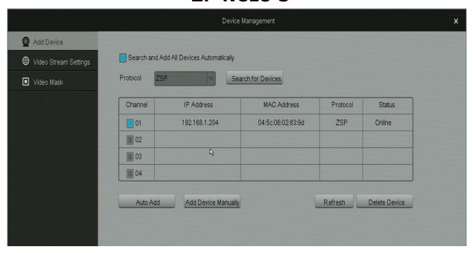
Here you can copy down the IP addresses and see which channels thay are currently connected to. Select the camera you wish to change using the box under "channel" and delete the cameras as needed. You can then select "ADD DEVICE MANUALLY"
