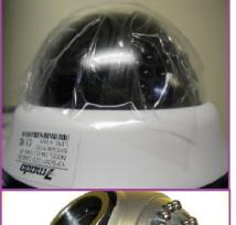
To remove the clear plastic dome cover, simply anchor the bottom plate of the camera and gently twist the white plastic section counter-clockwise.
