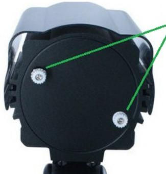
Once the rounded back cover has been removed from the camera, you will see two knobs located on the back of the camera. By rotating these two knobs, you will be able to adjust the zoom and the focus of this camera.
