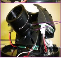
Once the camera's chipset is revealed, you can adjust the focus and the zoom by turning the two small black knobs that are directly attached to the lens.
