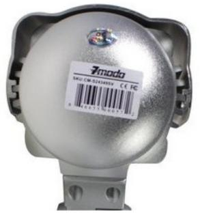
First, un-screw the rounded back cover from the back of the camera. This cover hides and protects the camera's vari-focal knobs.
