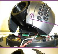
Removing the clear plastic dome cover will reveal the LED Ir light board and the camera's chipset.
