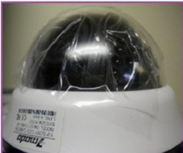
To remove the clear plastic dome cover, simply anchor the bottom plate of the camera and gently twist the white plastic section counter-clockwise.
