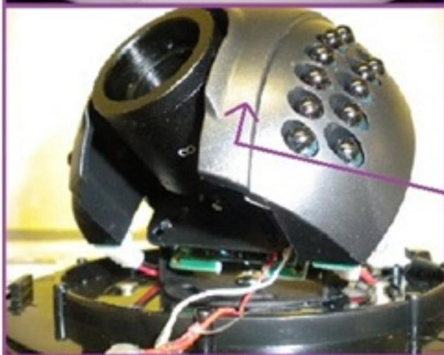
Removing the clear plastic dome cover will reveal the LED IR light board and the camera's chipset.
