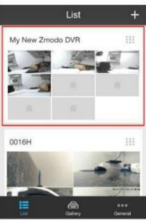
7. Select your system from the device list to view the live video stream. Go back to the 'Device List' section and select your device from the list. Make sure that a live video stream from your DVR appears.
