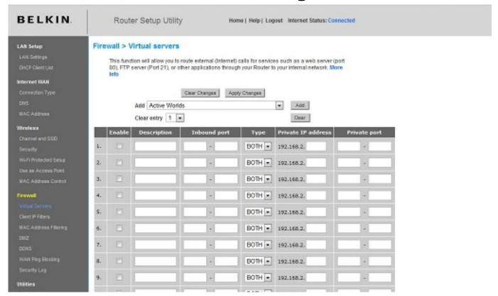
For Belkin routers, access port fowarding under Firewall, Virtual Servers. Be sure to check the 'Enable' box, then hit the 'Set' button, and save your changes.
