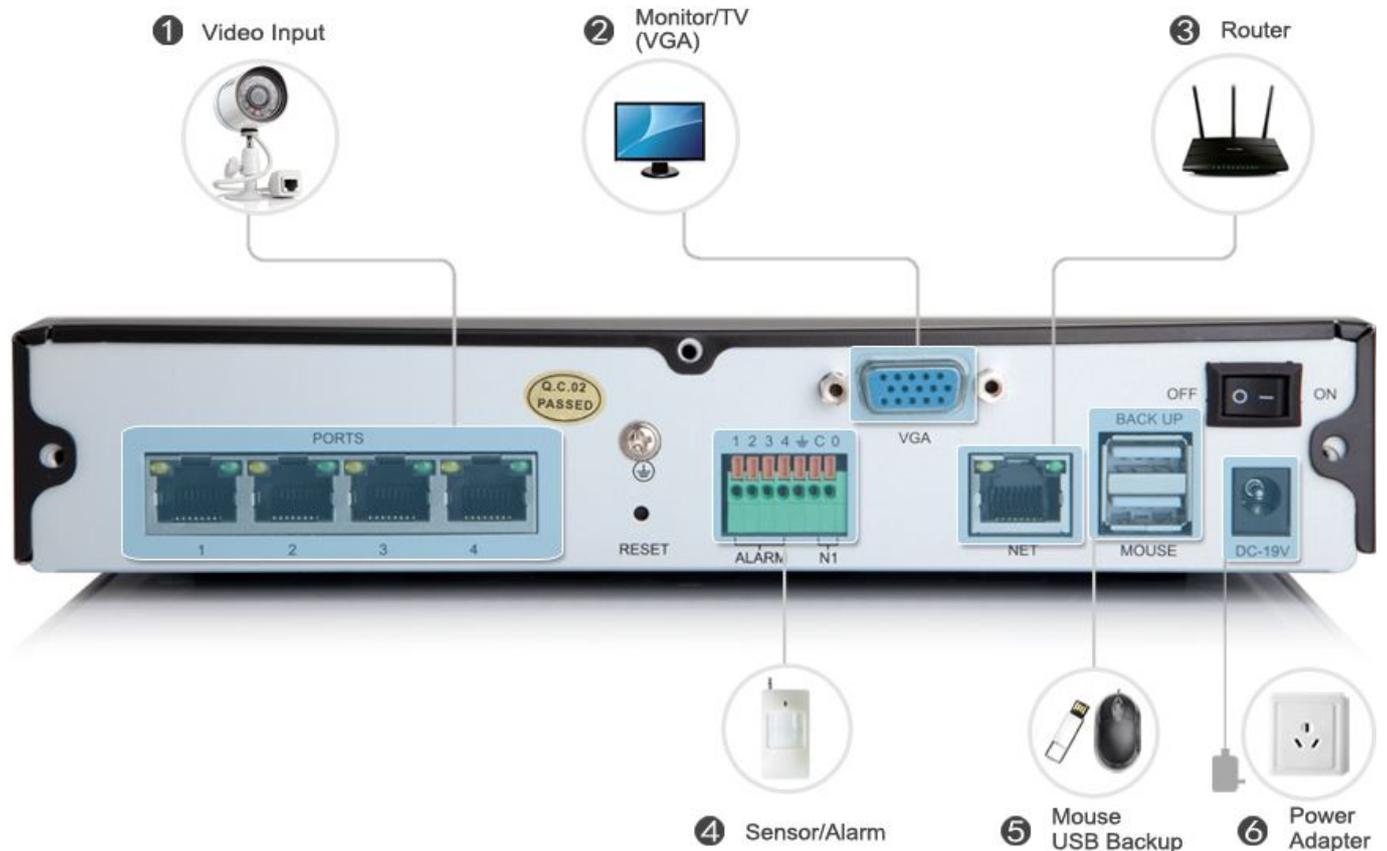
1. Make sure that your router is securely connected to the NET port on the NVR (ZP-NE14-S) using an ethernet cable. The NVR will be unable to locate the any cameras that are connected to it unless the NVR is also connected to a router.
