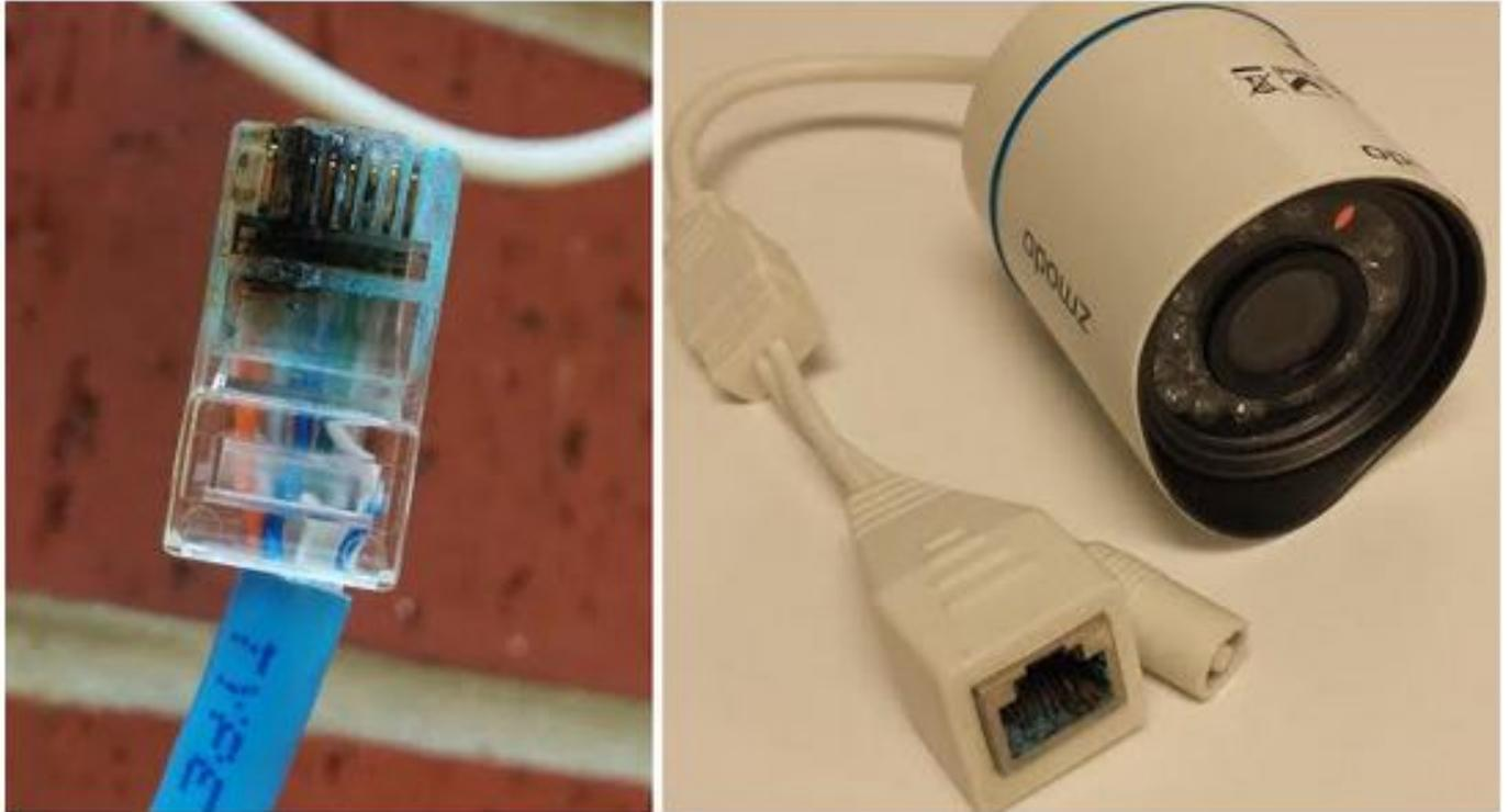
To weatherproof the cable ends, you can either tape the cable ends or install the cable ends into a conduit box. By far the safest option is to install the cable ends into a conduit box to protect the cable ends from the rain and wind.
