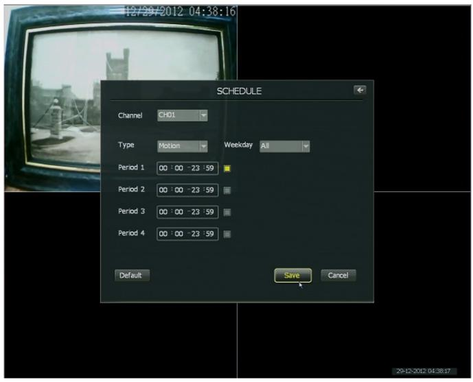
g. From the Motion Tab (accessed by selecting "Motion" in the drop-down box) set the time range to 00:00 - 23:59 in the Period1 field. Enable Period1 by selecting its check-box. This will enable motion recording.
