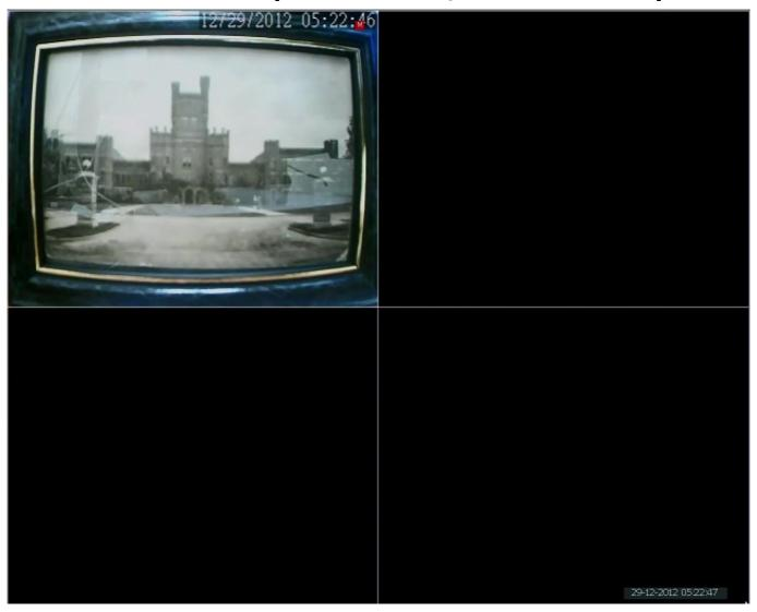
4. After saving those changes, exit out to the camera grid. When one of the cameras detects motion, the NVR will display a red M on the screen as it records for the duration of time that motion takes place.
