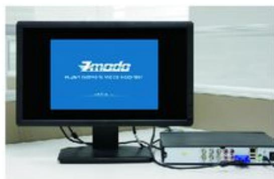
\* The ZMD-DD-SBN8 model has 8 channel inputs for cameras, and the ZMD-DD-SBN4 has 4 channel inputs for cameras.
