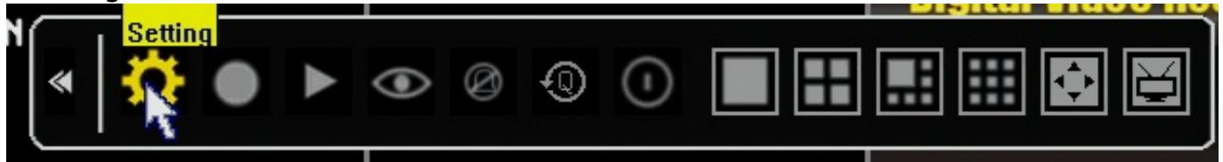
After entering the "Settings" menu, you will be on the System tab in the menu. You will need to click the Maintenance tab at the top. From the maintenance tab, you will click the star on the third line down marked "HDD MANAGE"
