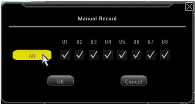
You should now have continuous record on all channels indicated by a grey/black dot in the top right of each camera window. This will record constantly as long as the DVR is turned on or until manual record is removed. If at any point you want to adjust the DVR to a more specific recording schedule you will need to disable manual record for the schedule to take over.
