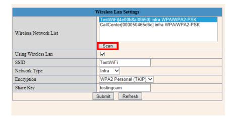
16. Type your WiFi password in the "Share Key" field and then click submit. The screen will change and start a 30 second countdown. Remove the ethernet cable with 20-25 seconds left.
