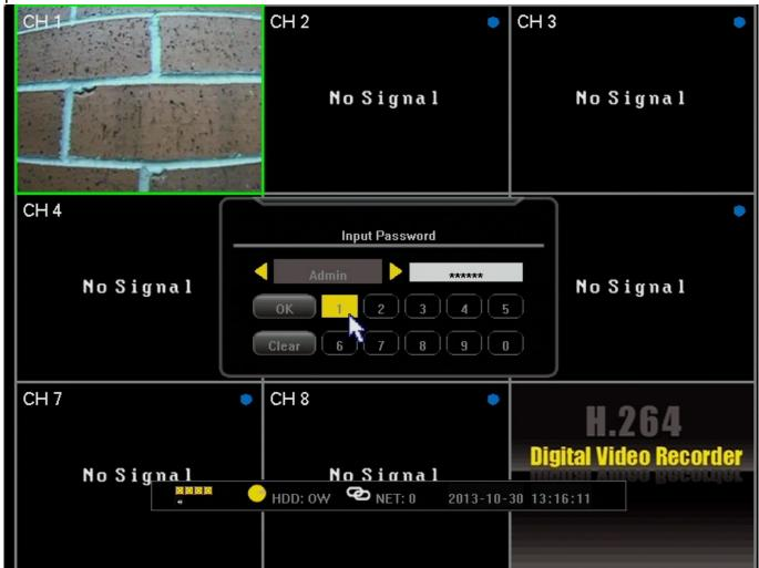
After logging in, right-click the mouse 2 times to bring up the toolbar along the bottom. From this toolbar select the far left icon that looks like a gear and says "Settings" when the mouse is over the icon.
