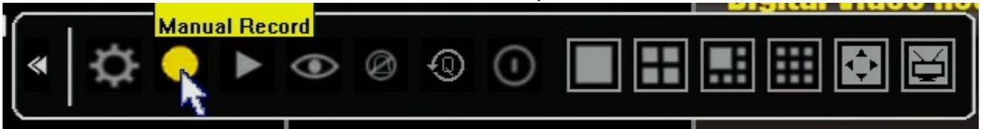
When you've selected Manual Record you will be given the window below. Hit the "All" button until all the check marks are removed from the boxes and hit ok. Manual record will now be disabled and the DVR will revert to the recording schedule you set in the menu. You are now finished and recording on motion and should be able to verify with the marks shown earlier.
