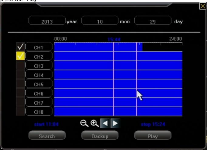
After pressing play you will be taken in to your video for the selected channels. Your video controls will be along the bottom. Controls include Rewind, Pause, and Fast forward. Pressing the stop button will take you back to the video search screen.
