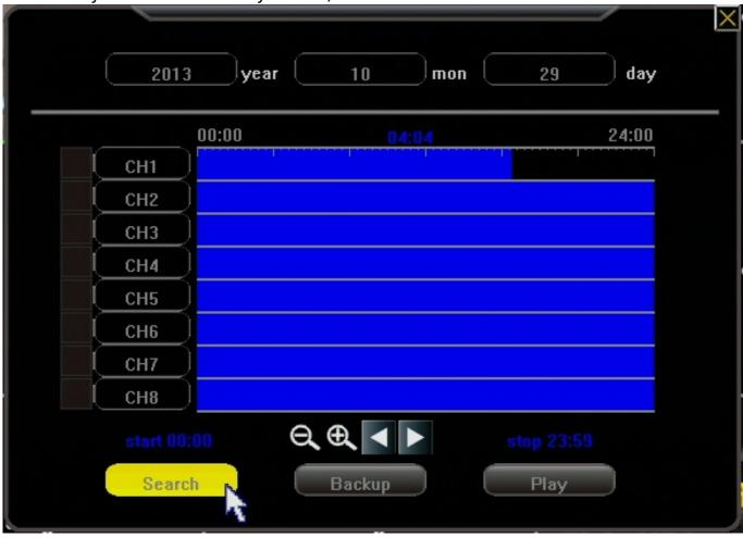
After the desired day has been set and you have clicked search the grid in the middle will have the video for that 24 hour period loaded in to it. From left to right the grid goes from midnight(start of day) to midnight(end of day). The horizontal bars are broken down by channel. In order to see video footage you will select a  $\frac{1}{2}$
