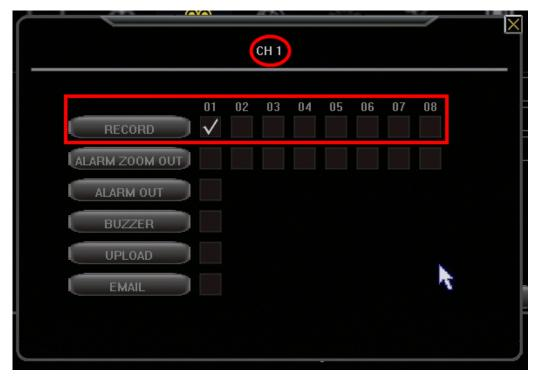
With these settings configured properly, you can have your DVR recording in specific time frames on motion detected in specific locations of your video feed.
