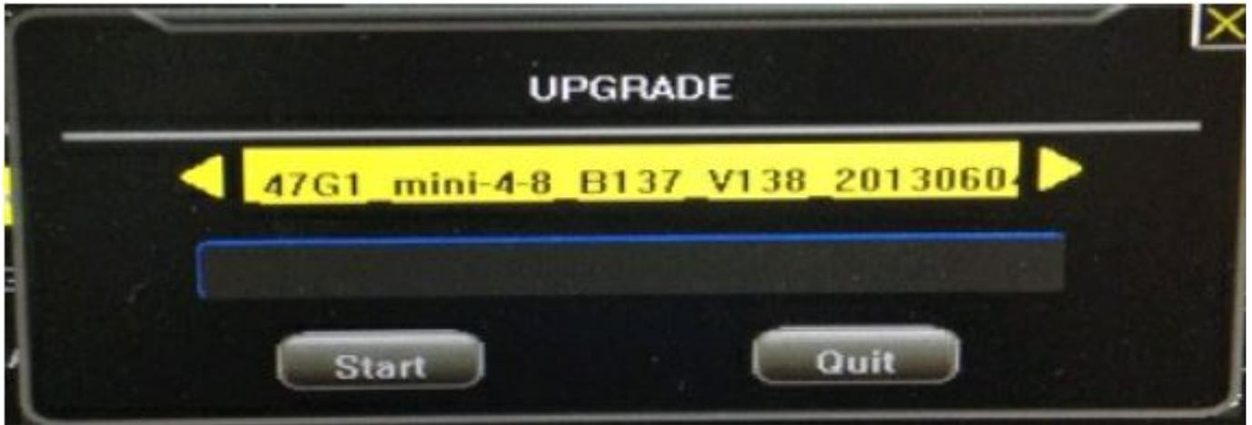
5. Select the appropriate upgrading firmware, based on your DVR model (4CH & 8CH DVRs use the same upgrading firmware), then click "Start". The upgrade will start (do not power off during the upgrade process);
