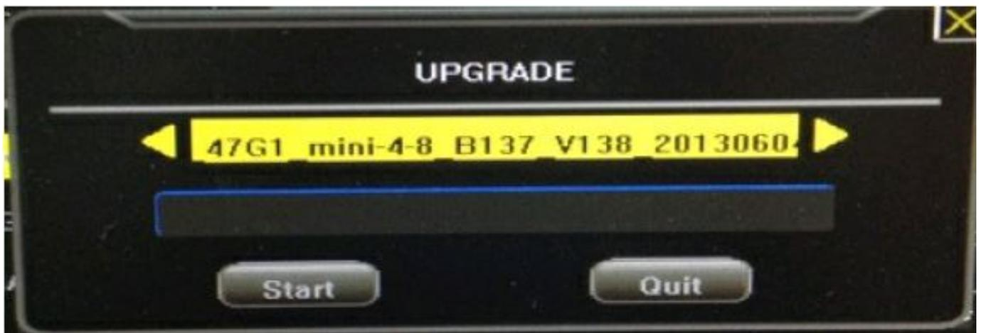
5. Select the appropriate upgrading firmware, based on your DVR model (4CH
