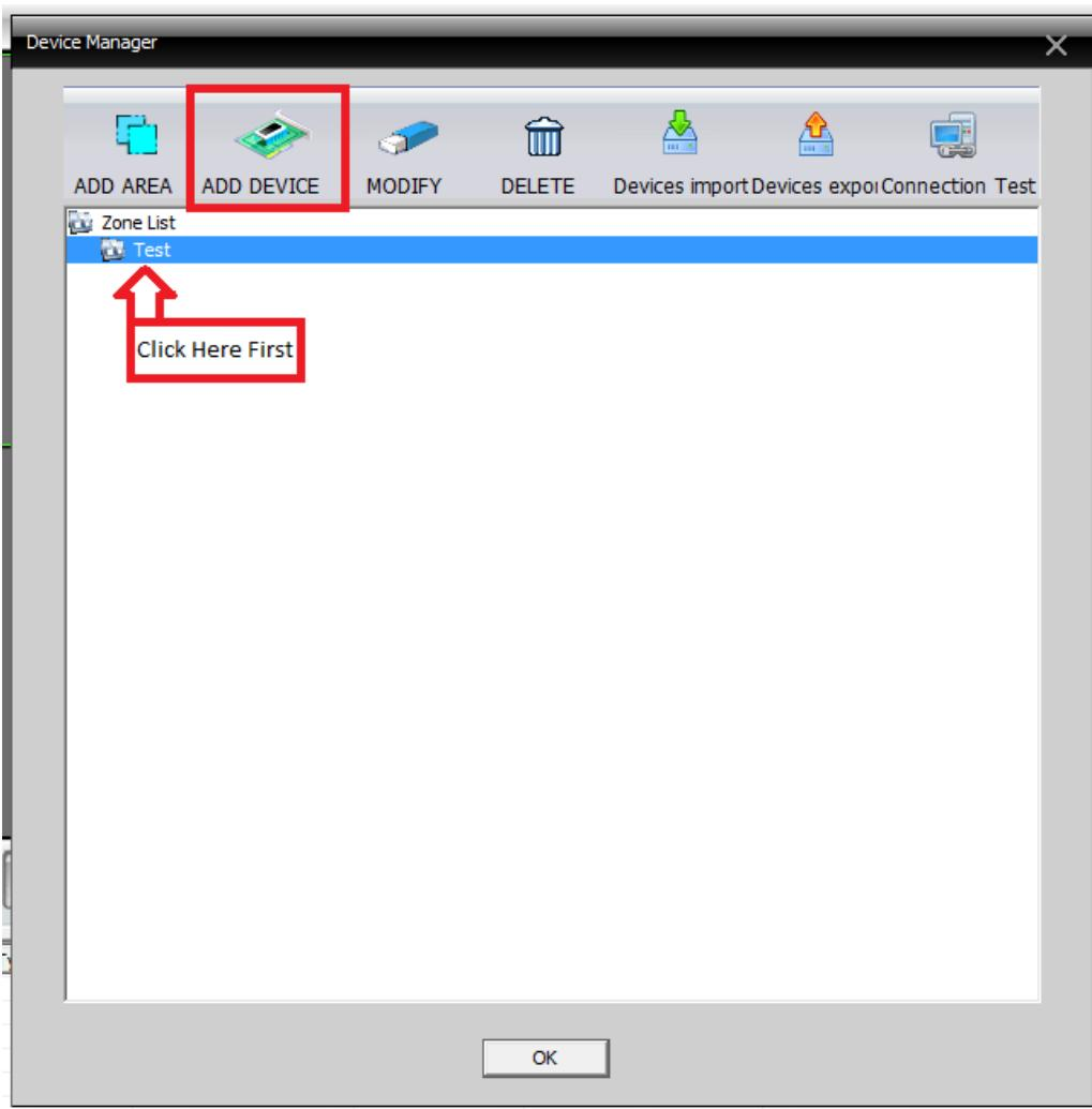
6. Before adding the new device, the DVR should already be setup for local or remote access. You will also need all the IP addresses, port numbers, and login information already setup on your DVR.
