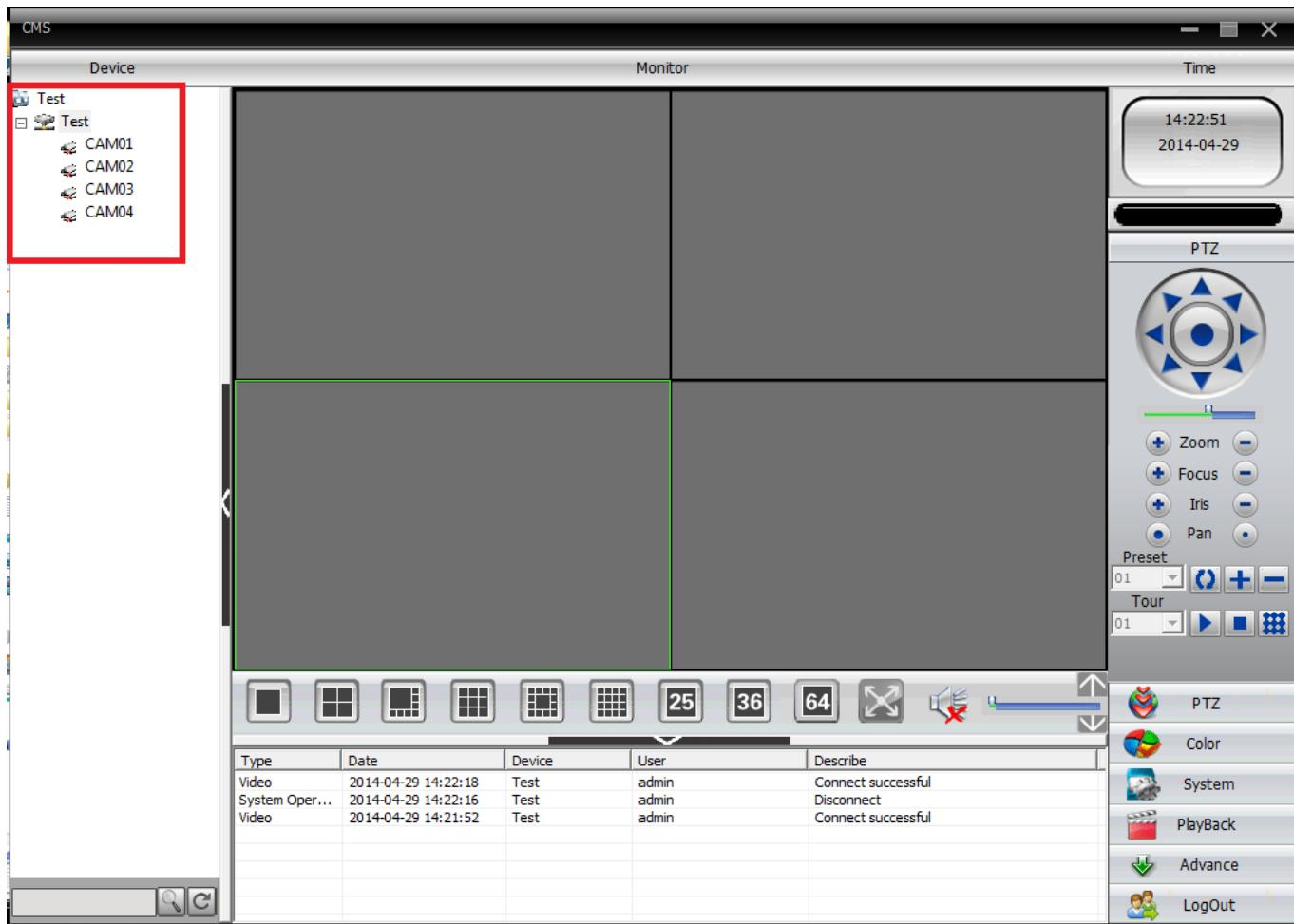
8. To connect to the cameras, right-click on the Device Name and select the option for **Connect all Video**.
