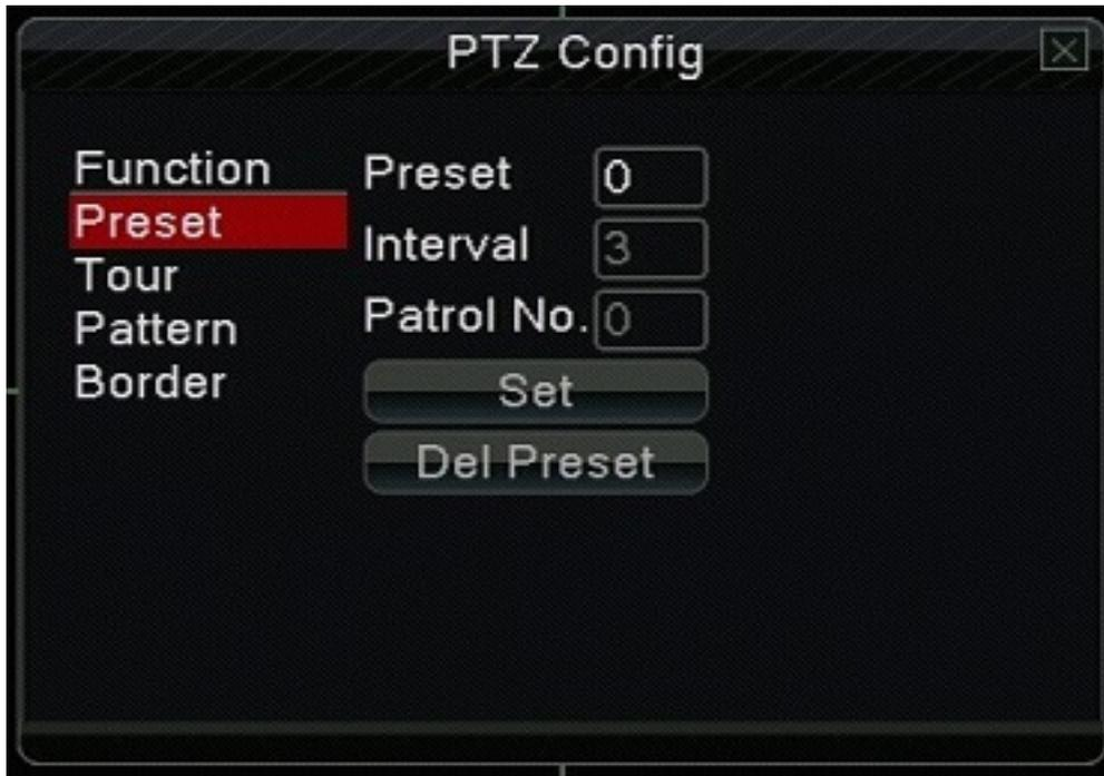
Click in the preset box and give a number to indicate the current position of the camera. Repeat using a different number for each preset position until you have all presets entered.
