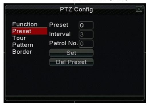
Click in the preset box and give a number to indicate the current position of the camera. Repeat using adifferent number for eace preset position until you have all presets entered.
