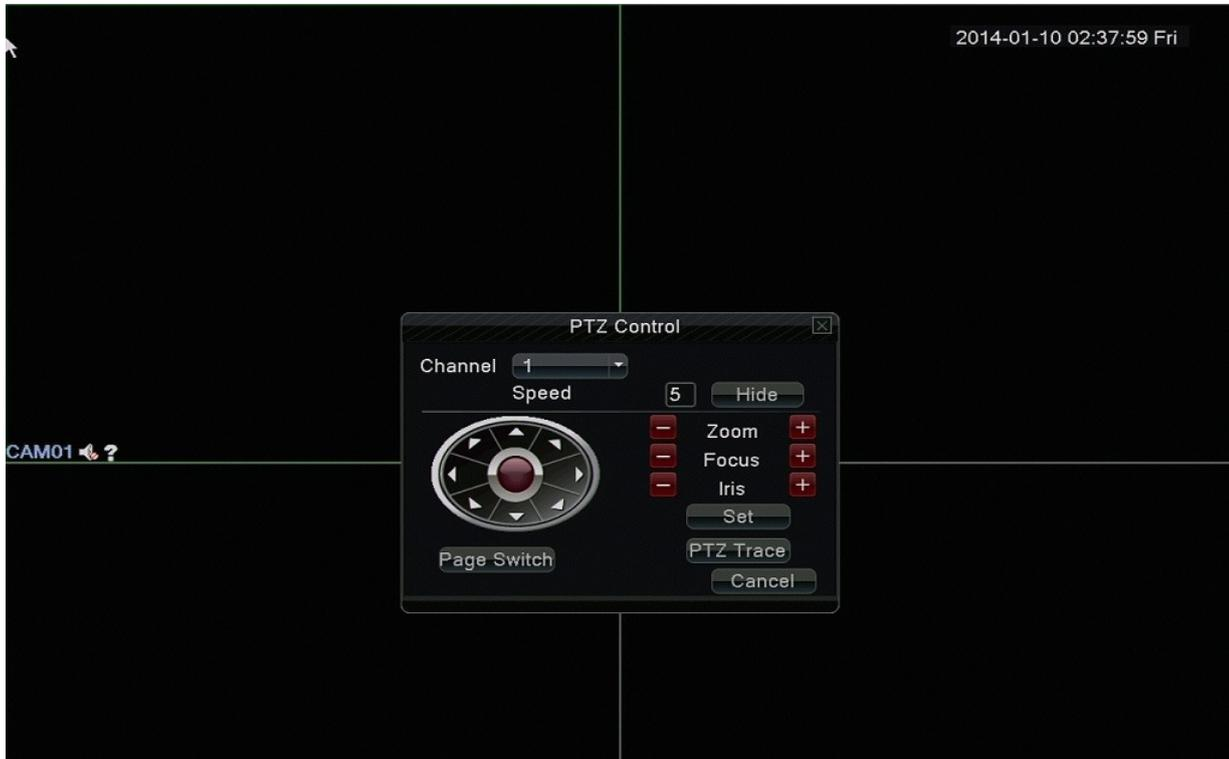
Step 2: Once you have the desired position, click Cruise buttons, then write proper value into the Cruise Line and Preset Points blank, then click "SET" which will open the PTZ Config menu.
