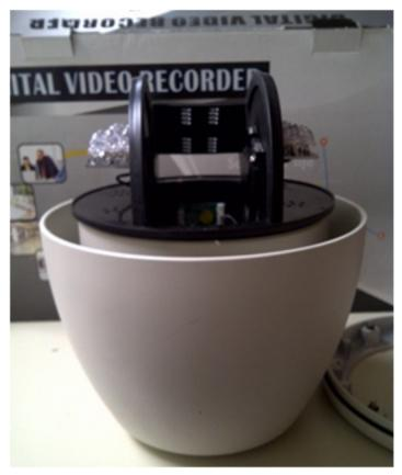
2. Once the inner housing appears to be completely seated and centered inside of the outerhousing, mount the outer housing cover just enough to hold the cover on.
