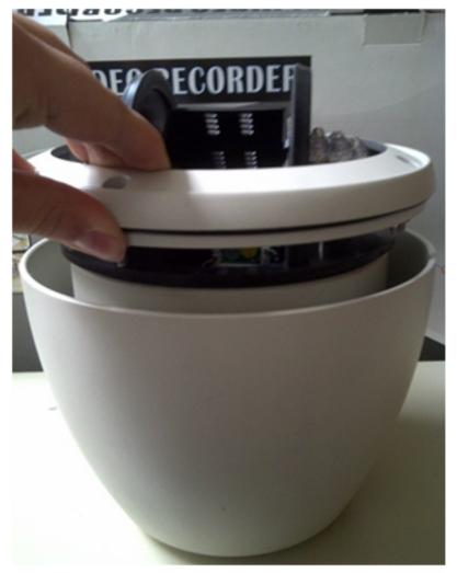
3. Now spin the dome. If there is resistance or a rubbing noise, take note of which side of the camera is causing the resistance. Remove the outer housing cover and slightly adjust the inner housing away from the areathat the rubbing occurred.
