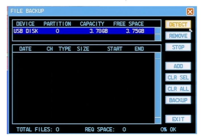
With your USB device now displayed on the screen select the "Add" button. This will bring up a search window almost identical to the playback window. This is shown below.
