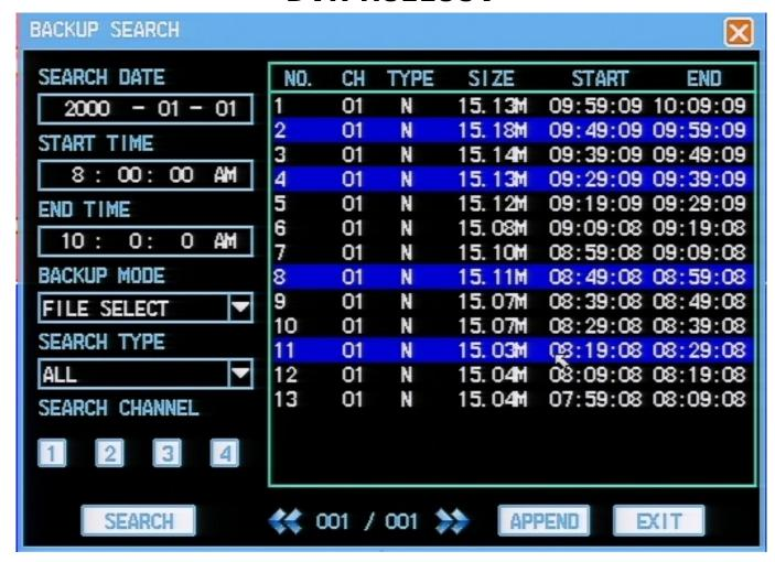
From top to bottom, in the backup search window, fill out the date, start time, and end time of the files you are looking for. Be sure to change backup mode to "File Select". You may narrow down the type of files returned with the search type(to display only files of regular record or motion record types).
