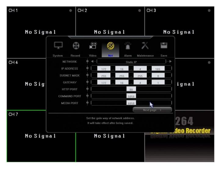
Set the Network to "Static IP" Enter the same information you entered into the adapter for IP, Subnet Mask and Gateway.
